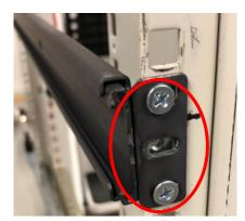
6. Push the lock upwards and forward to detach it from the rack assembly.
