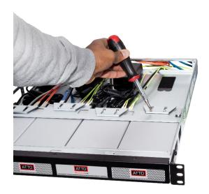
4. Mount the outer rail to the rack using bar nut and #10 32 3/8 flat head screws.
